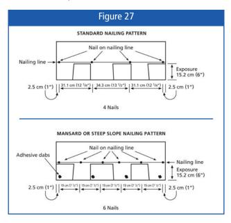
EVEREST and MYSTIQUE shingles offered in the East, must be nailed on the nailing line to allow penetration through the double-ply area just above the tops of the laminated tabs.
