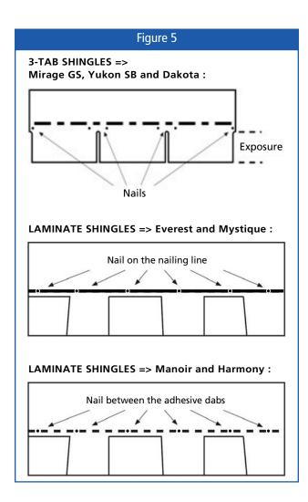
shingles must be fastened using 6 nails and all shingles located at the roof edges must be cement together in a 10 cm (4") wide layer of plastic cement. If above special application instructions are not followed, shingles will be warranted for winds from 115 km/h (70 mph) to 180 km/h (110 mph). See Table 1 for High Wind Warranty wind speed for the shingle being installed.
