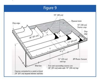
line. Beyond this point 91 cm (36"), sheets are laid, but without Asphalt Plastic Cement, lapping each course 48 cm (19") over the preceding one. Each course of felt is nailed sufficiently to hold it in place until the shingles are applied (see **Figure 9**).
