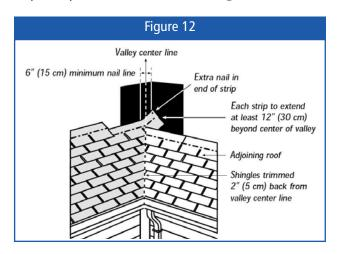
Installing a layer of GRIPGARD, GRIPGARD SX or PROGARD ULTRA Waterproofing Membrane in the valley, instead of roll roofing will ensure maximum protection.
