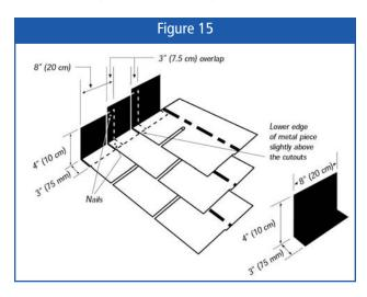
In re-roofing (application over an existing layer of shingles), ensure that the old shingles butting the wall are in good condition. Apply a strip of BP Smooth Surface Roll Roofing 20 cm (8") wide over the shingles along the wall. Nail 10 cm (4") apart along each edge of the strip. Cover with Asphalt Plastic Cement and embed the new shingles. Use a caulking gun and draw a bead of Asphalt Plastic Cement between the ends of the shingles and the siding.
