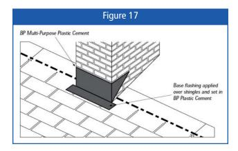
edges to permit folding up the sides of the chimney. Use MINI-PROGARD, GRIPGARD, GRIPGARD SX or PROGARD ULTRA Waterproofing Membrane as a super base for the flashing material. Extend 25 cm (10") up the chimney and onto the roof to the top of the cut-outs of the last shingle course. Secure this strip to the shingles with Asphalt Plastic Cement.
