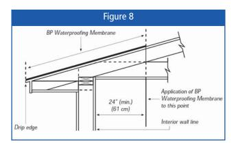
felt is nailed towards its upper edge with only enough nails to hold it in place until the shingles are applied (see Figure 8).
