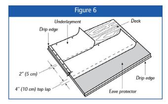
Nail sufficiently to hold the underlayment in place until the shingles are applied. Install shingles as soon as possible after installation of the underlayment. Building Products of Canada Corp. recommends installing the shingles the same day as the underlayment, to keep
