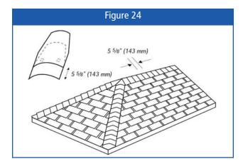
Nail cap with one nail on each side 15,2 cm (6") from the exposed end and 2,5 cm (1") from each side. The same method applies for the hip and ridges.
